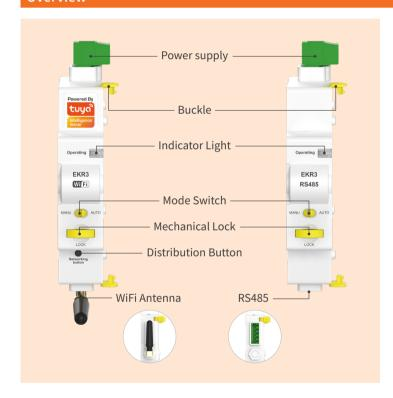
EKR3 smart MCB provides not only overload and short-circuit protection like traditional circuit breakers, but also the ability to remotely control the closing and timing of the MCB through the Tuya APP or RS485 platform, as well as obtain the switch status of the device.
